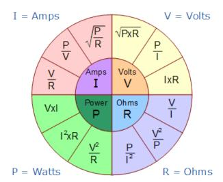
Ohm's law states that the current through a conductor between two points is directly proportional to the voltage across the two points. Introducing the constant of proportionality, the resistance, one arrives at the usual mathematical equation that describes this relationship;
