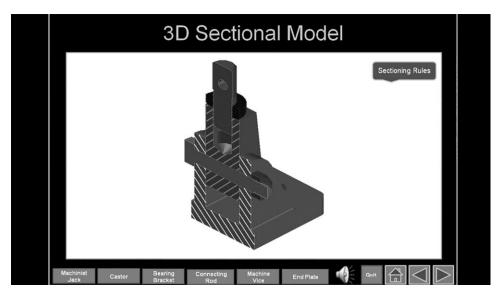
Figure 5. Shows a view of the 3 D sectional model of the machinist's jack
