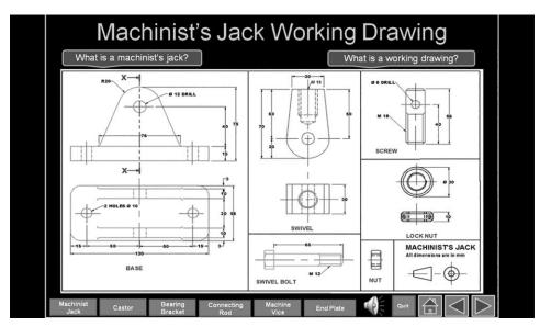
Figure 1. Shows the working drawing of the parts that make up the machinist's jack
