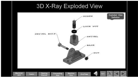
Figure 2. Shows the exploded view of the machinist's jack
