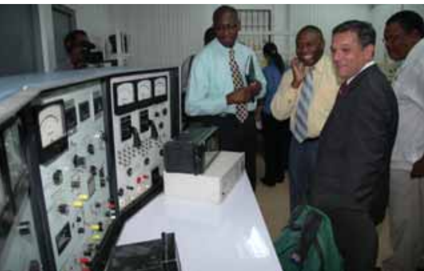
Mr. Damian Obiglio (right) shares a laugh with from left, Mr. Andrew Isaacs, Lecturer, School of Engineering, Mr. Ricardo Rennals, Director of Transmission, JPSCo. and Dr. Victor Watt, Head, School of Engineering as they examine the Multi-Amp Relay Test Set machine located inside the JPSCo Power Lab. The machine is used to calibrate and test relays used in electrical power systems.
