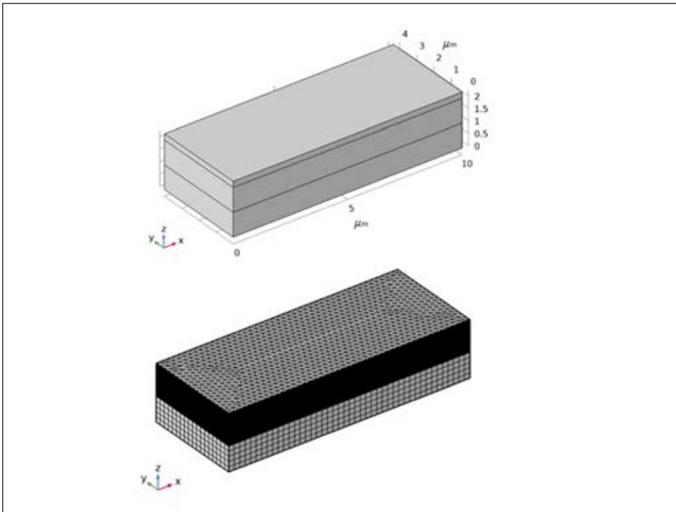
**Figure 1:** Geometry, dimensions, and mesh of the heterojunction wafer
