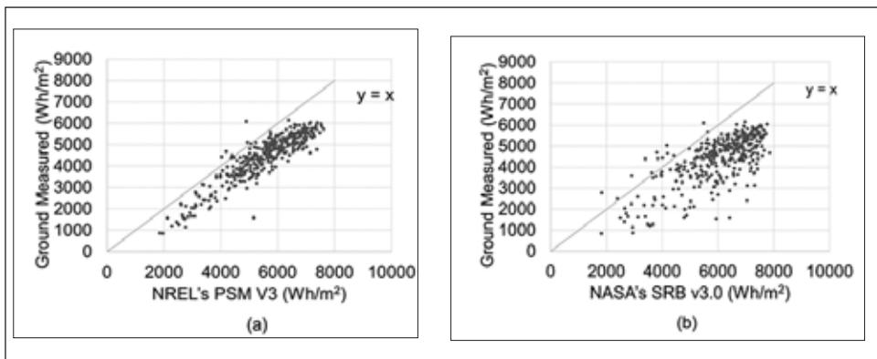
**Figure 1:** Scatterplots of the daily ground measured GHI totals compared to the modelled datasets for the year 2003
